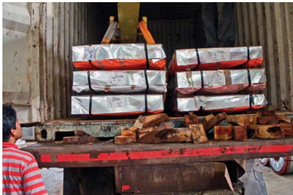
The steel is packed with corrugated material, which is covered with one layer of galvanising sheet and is then covered by a plastic material.
